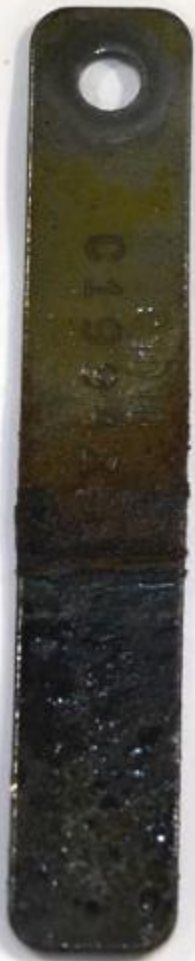
Steel Coupon Compressed Air
