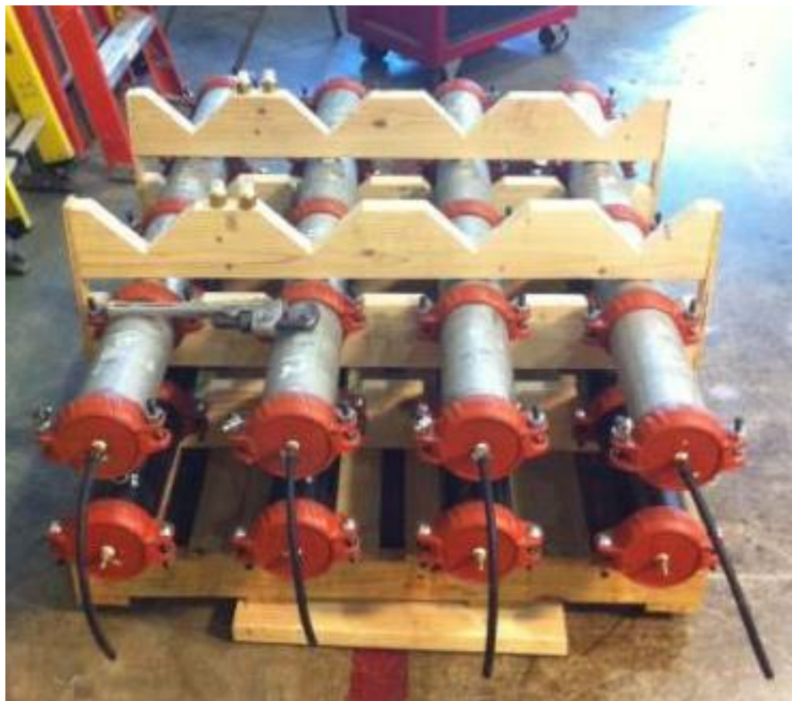
Corrosion Comparison Tests (0.010" Leak Diameter)
