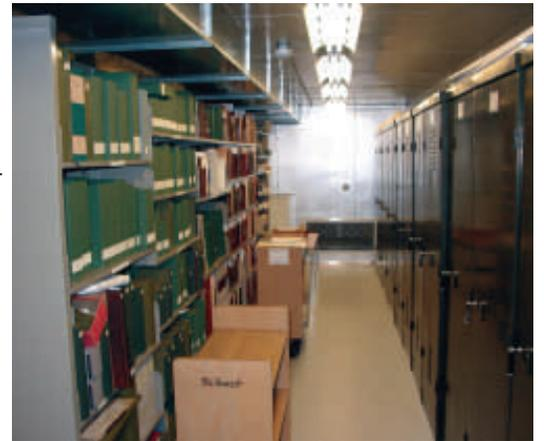
*Photo: Joe Arnold, Computer Environments, Livonia, Mich., and Dectron Internationale, Roswell, Ga. | The original prefabricated room envelope that contains the papyrus collection, which consisted of metal skin walls with an excellent R-15 insulation value, was still in mint condition and didn't need updating during the indoor air quality retrofit.*
